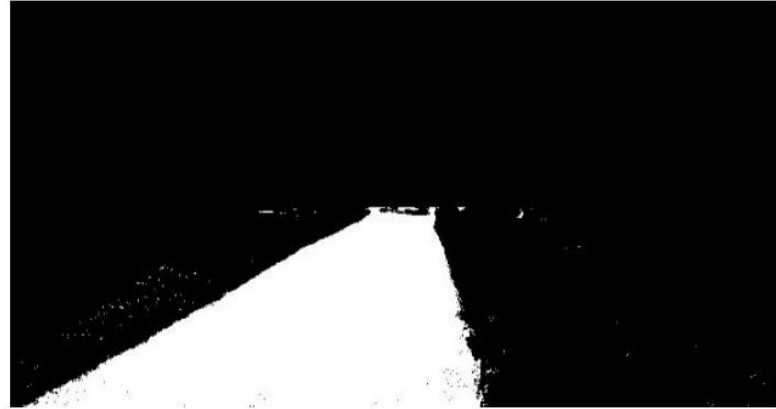
Fig12: The detected road surface
